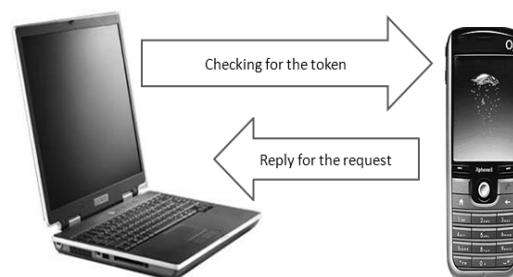
Fig. 1.5 Connection and Disconnection: Laptop checking for mobile phone presence.
