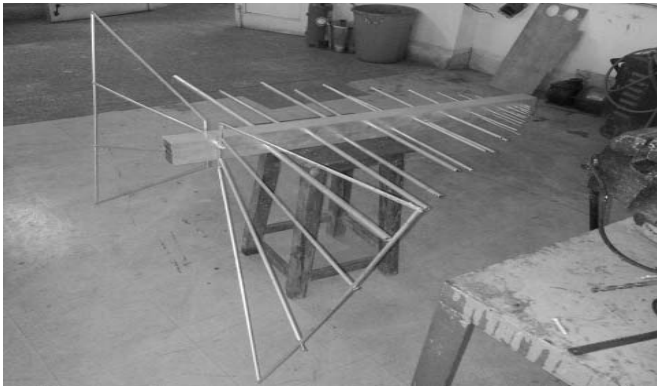
Fig.7 Practical Implementation of the designed antenna
