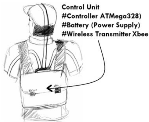
Fig.2 Position of Sensors, Xbee, Controller, Battery at user side
