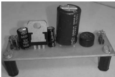
Fig. 4 Power Supply Module
