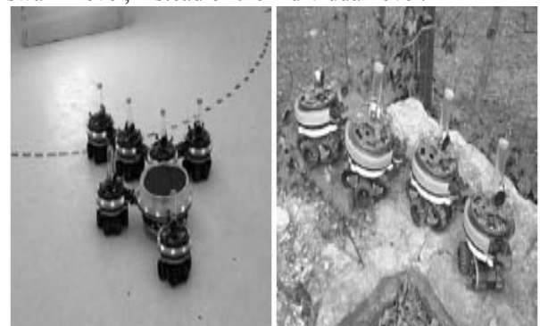
Fig.2 : Left: 6 S-bots, of which 4 in Swarm Robot formation, collaborate to transport a heavy object. Right: A 4 S-bots linear Swarm Robot moves on rough terrain.
