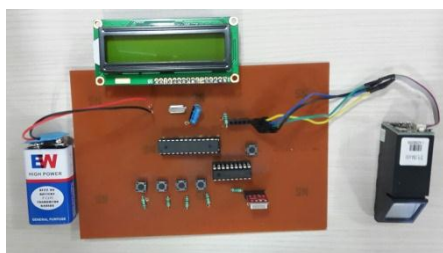
Figure 3: Module to enroll the user (Virtual SIM)
