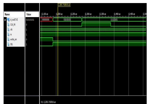
Fig 8: Data stored in RAM
