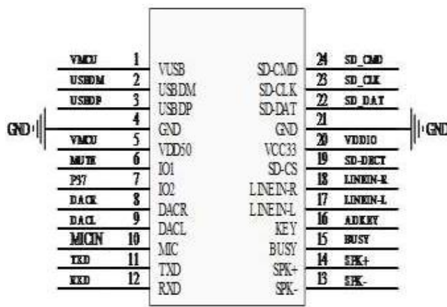
Fig.5 : Pin Configuration of FN-4M01(MP3 Player)
