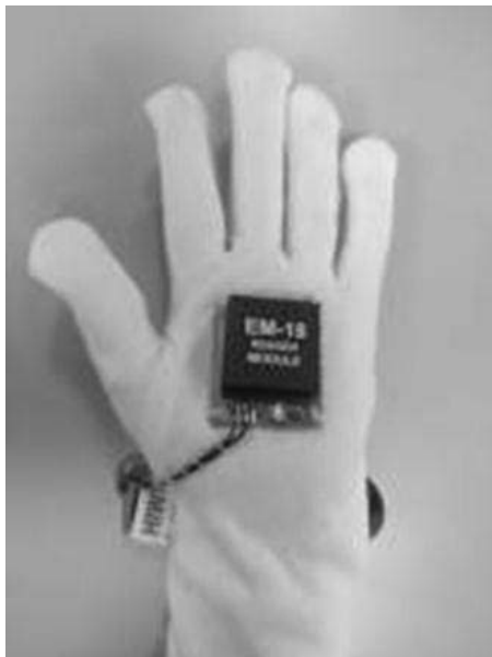
Fig 2.1: RFID Glove (back view) Scanning an R-Tag
